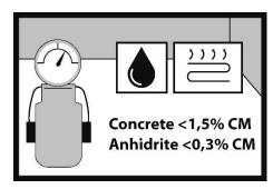
If the SPC panels are installed on an underfloor heating system, the moisture content (humidity) should not exceed 1.5% for concrete subfloor and 0.3% for anhydrite subfloor. The measurement results should be documented.
