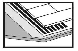
The limit above which the heating system should not be set is 27°C on the panel surface. The screed moisture content for installation on an underfloor heating system should not exceed: 1.5% CM for cement screeds, 0.3% CM for anhydrite screeds.
