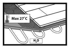
To avoid uneven operation of the panel core, the entire floor surface should be heated. If there are two or more heating loops in one room, the set temperature difference between the loops must not exceed 5°C. This also guarantees the greatest comfort of use (no colder spots on the floor surface).
