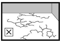
The subfloor should be dry, stable without scratches and cracks and clean without visible dirt. Fill cracks and defects in cement or anhydrite subfloor with filler. For floating installation on ceramic tiles, fill joints with a width of more than 5 mm and a depth of 2 mm with filler. For adhesive installation, fill all joints with putty and read the adhesive system manufacturer's guidelines.
