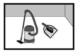
Brush or vacuum clean the subfloor before installing the SPC panels. The subfloor should be free of dust, debris, paints, varnishes, wax, grease, oil, hardeners, sealants, solvents, sand, glue residues, fats and other foreign bodies.
