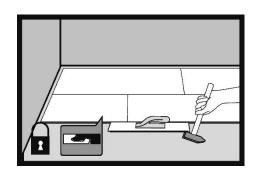
Use the tapping block to tap the long side of the panel. When installing the panels, always tap the joints on the long side of the panel.
