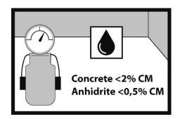
The moisture content (humidity) of the wooden subfloor (or wood-based boards) should not exceed 12%. The moisture content (humidity) should not exceed 2% for concrete subfloor and 0.5% for anhydrite subfloor. The measurement results should be documented.
