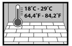
The temperature in the room where the floor is installed should be between +18°C and +29°C.
