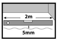
The maximum permissible unevenness is up to 5 mm, measured over a length of 2 m. Spot/local unevenness must not exceed 2 mm over a length of 1 m.
