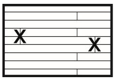
A natural floor layout can be achieved by mixing panels of different lengths in one row of panels. The minimum recommended shift of the joints on the short edges of the SPC panels in adjacent rows of panels must be greater than 200 mm.
