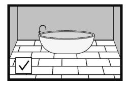
The SPC panels with integrated underlay can be installed as floating floors in bathrooms and other rooms where water spills may occur. When installing the panels as a floating floor, it is necessary to leave an expansion gap with a width of at least 5 mm in the door frame. (suitable for the type of masking expansion gap strip). The expansion gap can be filled with an elastic filler). When installing the panels as a floating floor, always leave a perimeter expansion gap with a width of 5 mm.
