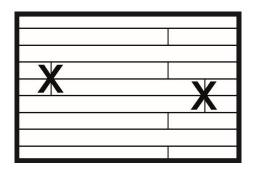
A natural floor layout can be achieved by mixing panels of different lengths in one row of panels. The minimum recommended shift of the joints on the short edges of the SPC panels in adjacent rows of panels must be greater than 200 mm.
