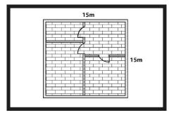
The maximum dimensions of the floor plan of a house/apartment for which the SPC floor installed as a floating floor does not require expansion gaps in doorways are 15m×15 m. For dimensions up to 15m x 15m do not make expansion gaps in doors and doorways to adjacent rooms. Make expansion gaps around walls and building elements such as stairs and columns.
