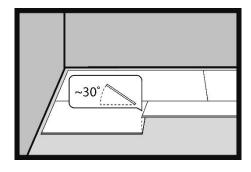
Use a hand saw or electric saw to cut the panels. When cutting the peripheral panels, remember to leave an expansion gap of at least 10 mm. The recommended length of the peripheral panel (A) in the first row of panels should be at least 200 mm. If the cut length of panel (B) is longer than 200 mm, you can use it to start laying the second row of panels. The distance between end-to-end joints in two adjacent rows of panels should be at least 200 mm.
